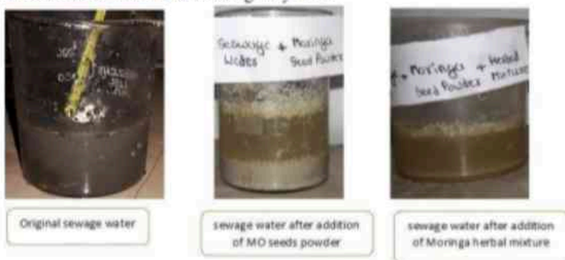
Fig.C- Shows effect of MO seed powder and its herbal mixture in sewage water
